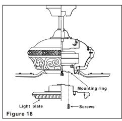
**REMEMBER:** To disconnect the power. The fan blades must be already attached to the fan.
