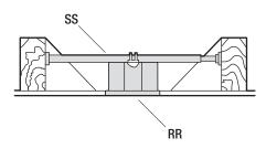
To hang your fan where there is an existing fixture but no ceiling joist, you may need an installation hanger bar (SS) (not included) as shown above.
