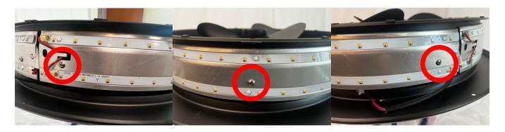
10. Unplug and remove and dispose of the defective LED strip
