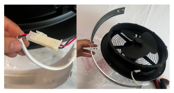
11. Bring the new replacement LED strip and connect the wire connectors.
