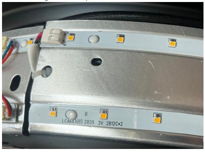
13. Insert and tighten all x3 removed LED strip screws.
