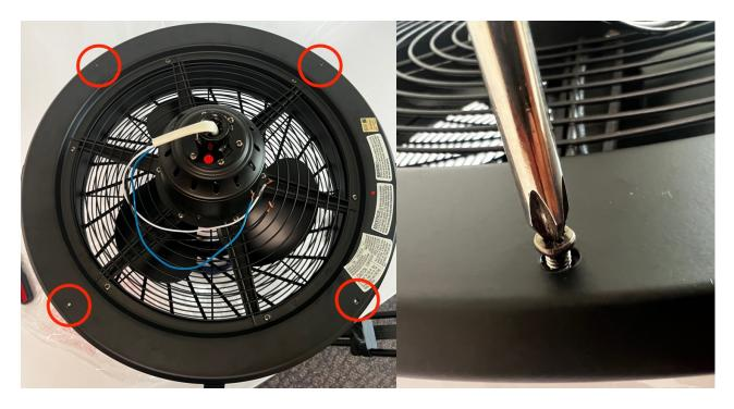
2. On the bottom of the motor, remove all x4 plastic screw covers. If difficult, use the point of a sharp knife.
