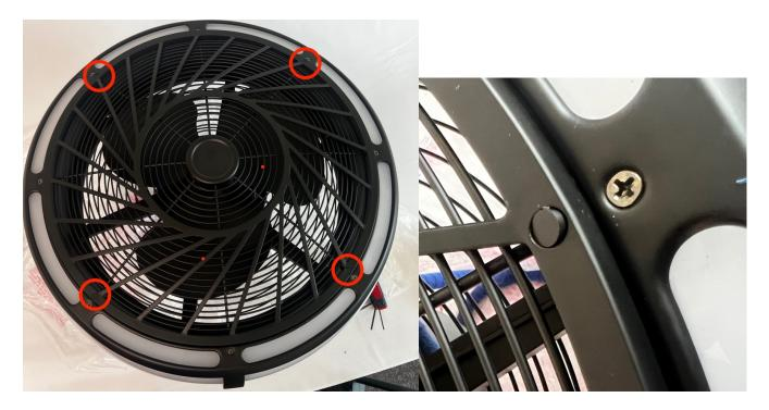
22. On top of the motor, insert and tighten all x4 removed outer housing screws.
