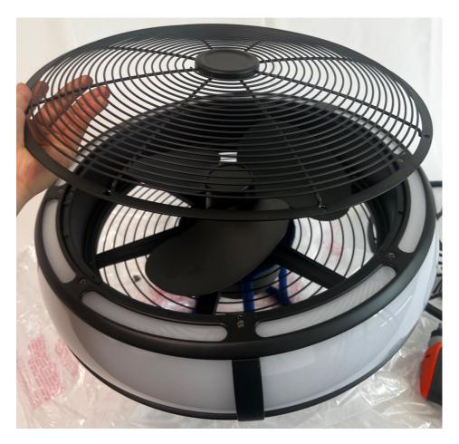
18. Insert and tighten x4 guard screws, being sure to leave a hole open between each screw.
