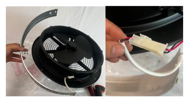
12. Align the LED strip holes with the screw holes on the motor.
