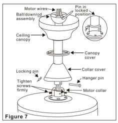
Make the Electric Connections WARNING: To avoid possible electrical shock, be sure electricity is turned off at the main fuse box before wiring.
