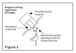
Note: You may need a longer downrod to maintain proper blade clearance when installing on asteep, sloped ceiling.
