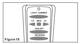
4. The "REV" button is used to set the fan forward or reverse, press the button forward (for warm weather) or reverse (for cool weather):
