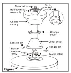
Make the Electric Connections WARNING: To avoid possible electrical shock, be sure electricity is turned off at the main fuse box before wiring.
