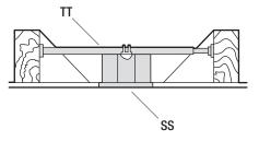
To hang your fan where there is an existing fixture but no ceiling joist, you may need an installation hanger bar (TT) (not included) as shown above.
