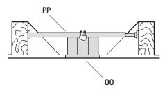
To hang your fan where there is an existing fixture but no ceiling joist, you may need an installation hanger bar (PP) (not included) as shown above.
