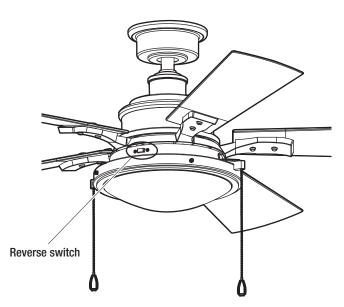
Warm weather - (Counterclockwise Direction) A downward air flow creates a cooling effect. This allows you to set your air conditioner on a warmer setting without affecting your comfort.
