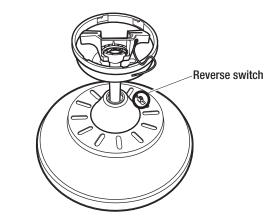
Warm weather - (Counterclockwise Direction) A downward air flow creates a cooling effect. This allows you to set your air conditioner on a warmer setting without affecting your comfort.
