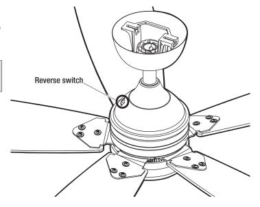
Warm weather - (Counterclockwise Direction) A downward air flow creates a cooling effect. This allows you to set your air conditioner on a warmer setting without affecting your comfort.
